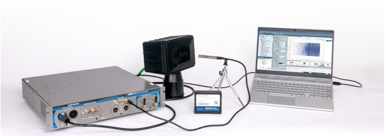
With the release of APx500 software version 7.0, Audio Precision adds support for GRAS SysCheck2-capable microphones, including the 246AE 1/2" CCP Free-Field Microphone Set pictured here. The combination of SysCheck2 and APx allows the user to verify the accuracy of the entire signal chain without physical access to the microphone or potential disruption of the test setup.
