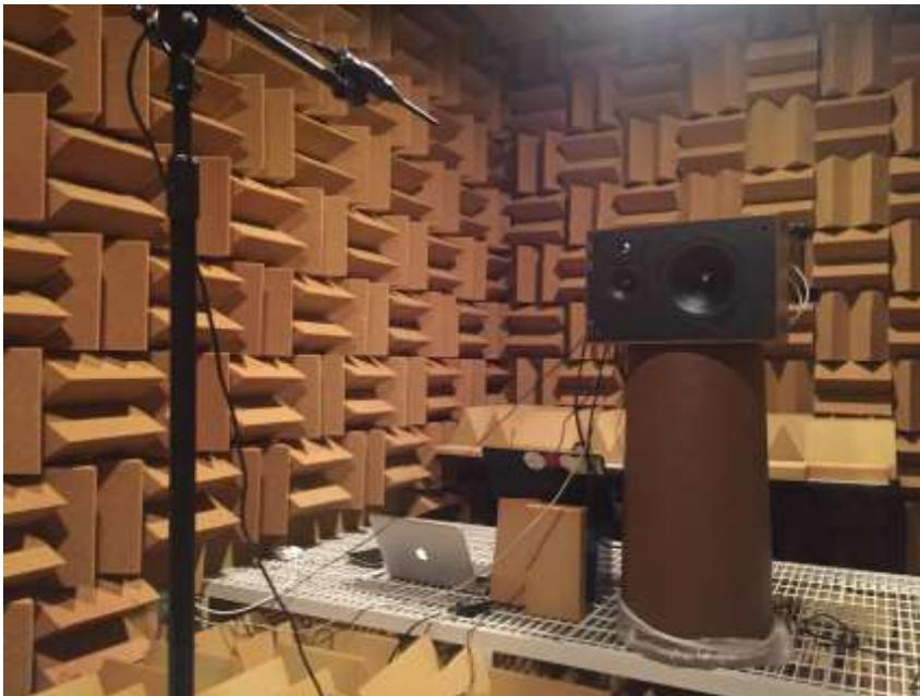
**Figure 2** The Test Setup Inside the Anechoic Chamber
