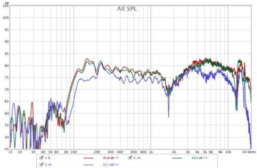
**Figure 6** 1929 Hz Crossover Frequency, Vertical Orientation.
