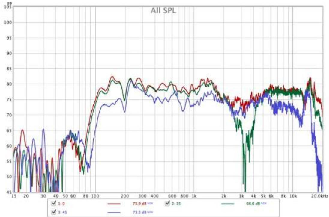
**Figure 3** 3850 Hz Crossover Measured at 0, 15, and 45 Degrees.
