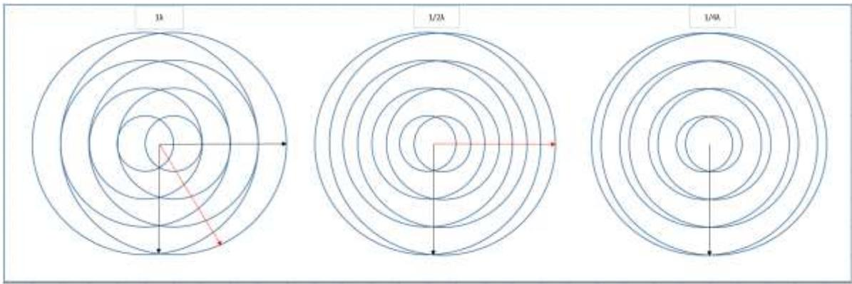
**Figure 1** Interference of Two Transducers at  $1$ ,  $\frac{1}{2}$ , and  $\frac{1}{4} \lambda$
