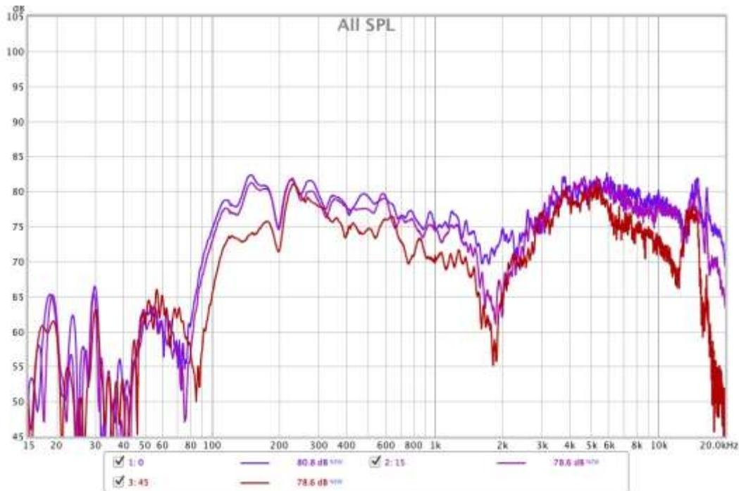
**Figure 4** 1929 Hz Crossover Measured at 0, 15, and 45 Degrees.
