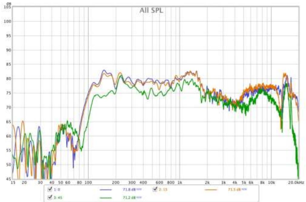
**Figure 5** 3850 Hz Crossover Frequency, Vertical Orientation.
